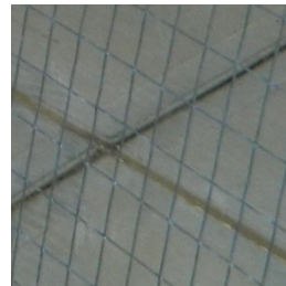
1" x 2" 14-gauge welded wire
